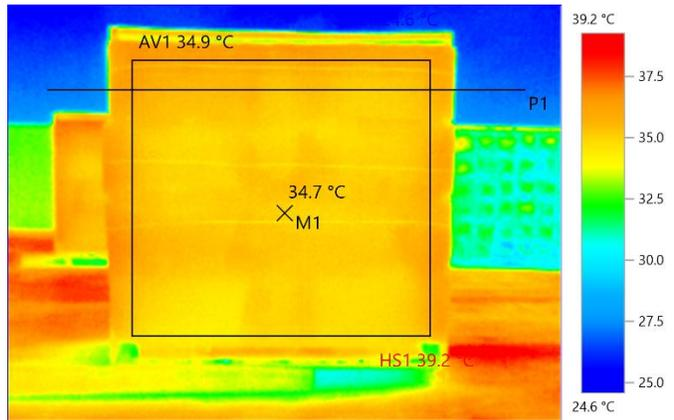
*Control Experiment: Temperature at Measuring Point 1 (M1) – 34.7°C, 15/08/2019, 12.00 p.m.*
