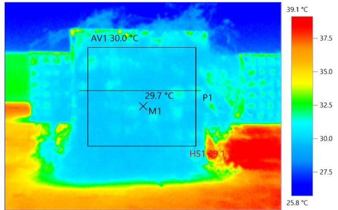
*Experiment A: Temperature at Measuring Point 1 (M1) – 29.7°C, 15/08/2019, 12.00 p.m.*
